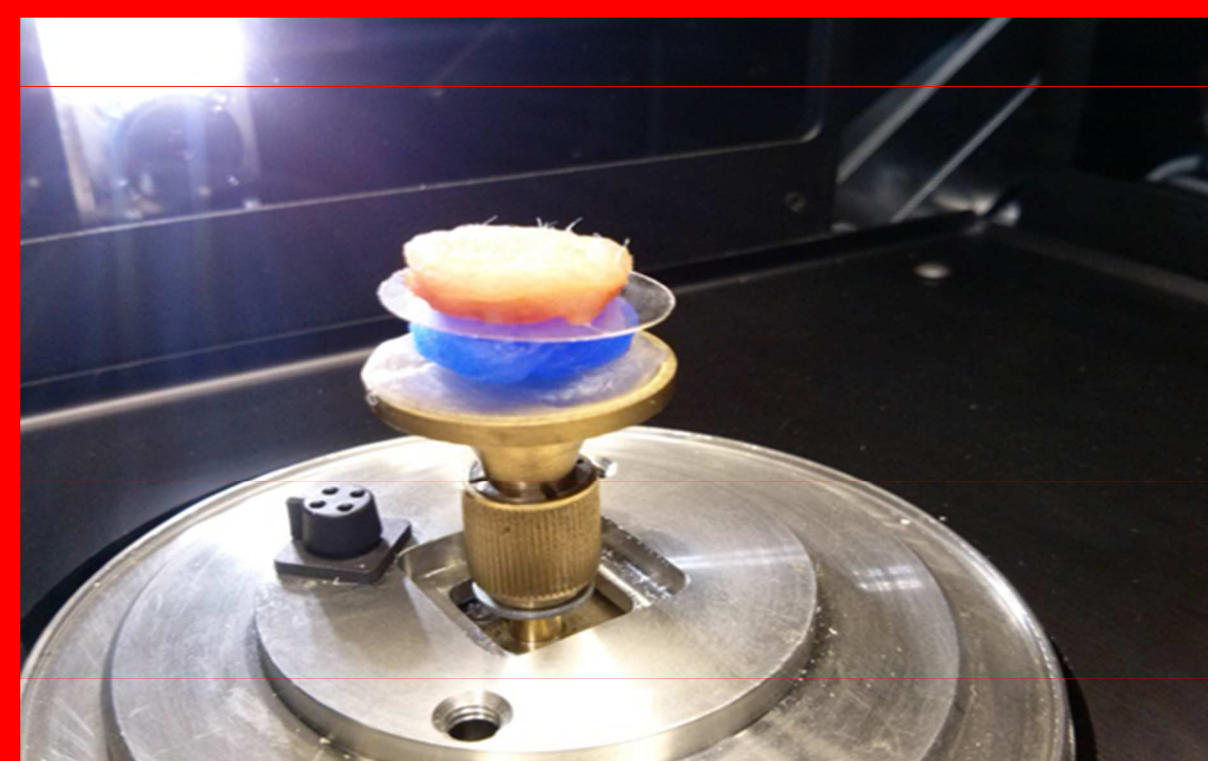
Fig. 3 Ex-vivo human skin in the SKYSCAN 1272 high-resolution micro-CT
